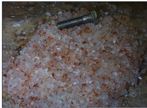
FIGURE 2 a) Typical response curve for coarse potash flotation using Eriez HydroFloat™ separator, b) Potash concentrate photo with 3/8-inch (9.5-mm) bolt shown for scale.
